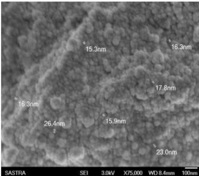
**Fig. 2:** FESEM image of 5% Mn doped ZnS nanoparticles
