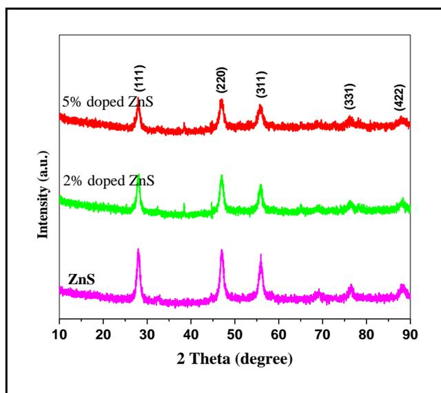
Fig. 1: XRD pattern of Mn doped ZnS nano particles
