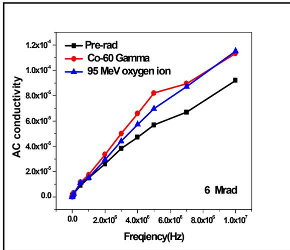
**Figure 5. Variation of ac conductivity versus frequency for unirradiated and irradiated LACC crystals (after 6 Mrad)**
