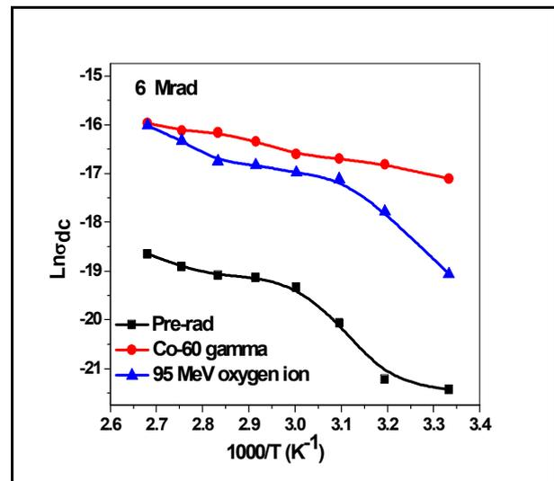
Figure 8. Plot of  $\ln\sigma_{dc}$  versus  $\frac{1000}{T}$  (K<sup>-1</sup>) for unirradiated and irradiated LACC crystal (after 6 Mrad)
