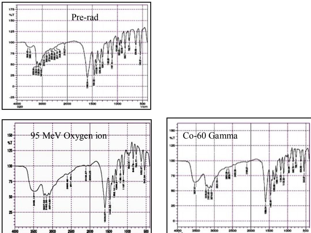
Figure. 2. FT-IR spectra of unirradiated and irradiated LACC crystals (after 6 Mrad)
