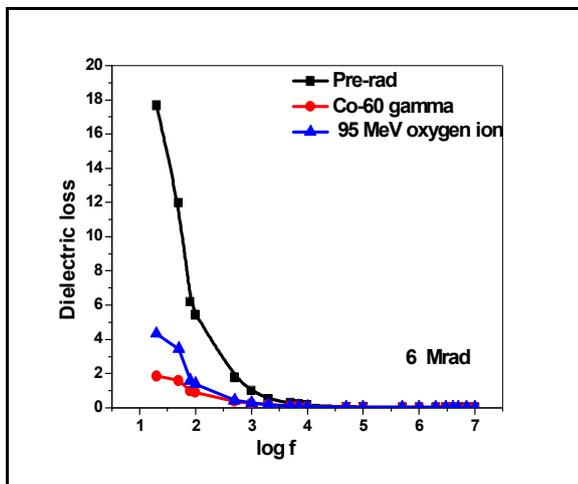
Figure 4. The Variation of dielectric loss as a function of frequency for unirradiated and irradiated LACC crystals (after 6 Mrad)
