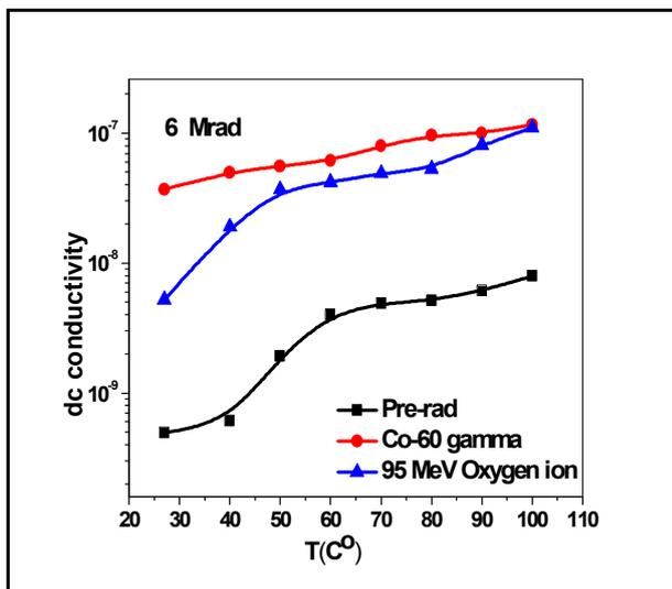
Figure 7. Variation of dc conductivity versus temperature for unirradiated and irradiated LACC crystal (after 6 Mrad)
