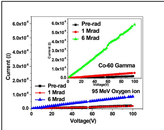
Figure.6. I-V graph of unirradiated and irradiated LACC crystals
