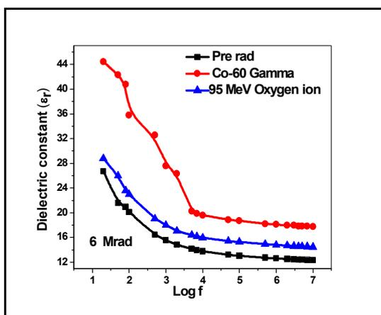
Figure 3. Plot of dielectric constant versus applied frequency for unirradiated and irradiated LACC crystals (after 6 Mrad)
